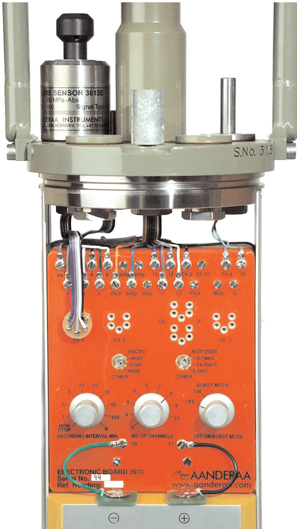
RCM11 Top end plate with a selection of sensors and wiring to the Electronic Board
