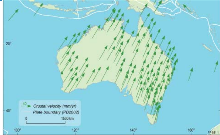
Figure 1. The difference between GDA94 and GDA2020 coordinates is primarily due to tectonic plate motion.
