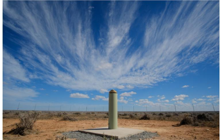
Figure 1. The new CORS basestation near Nullarbor, South Australia.
