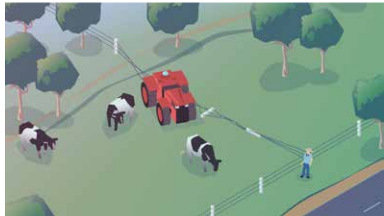
In 2020, a driverless tractor using satellite positioning to work a paddock mapped under GDA94 will need to know the paddock and its national coordinates have moved 1.8 m since GDA94 was established.
