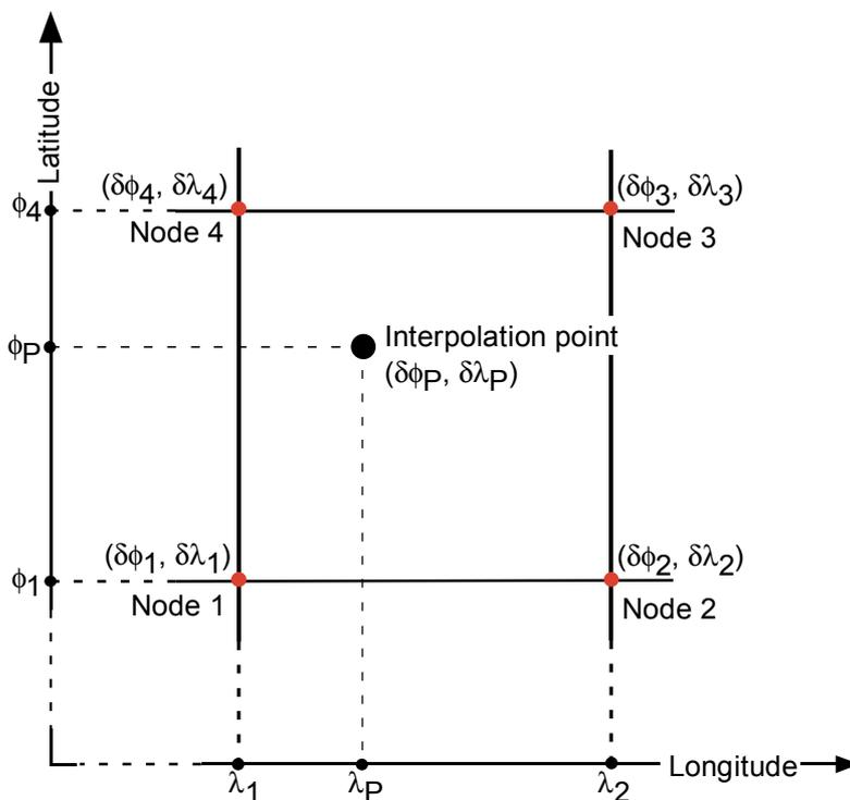
**Figure 1** – The principle of grid-based transformation
