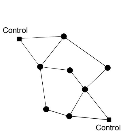
**Figure 2(a)** – Coordinates are calculated based on existing control and measurements
