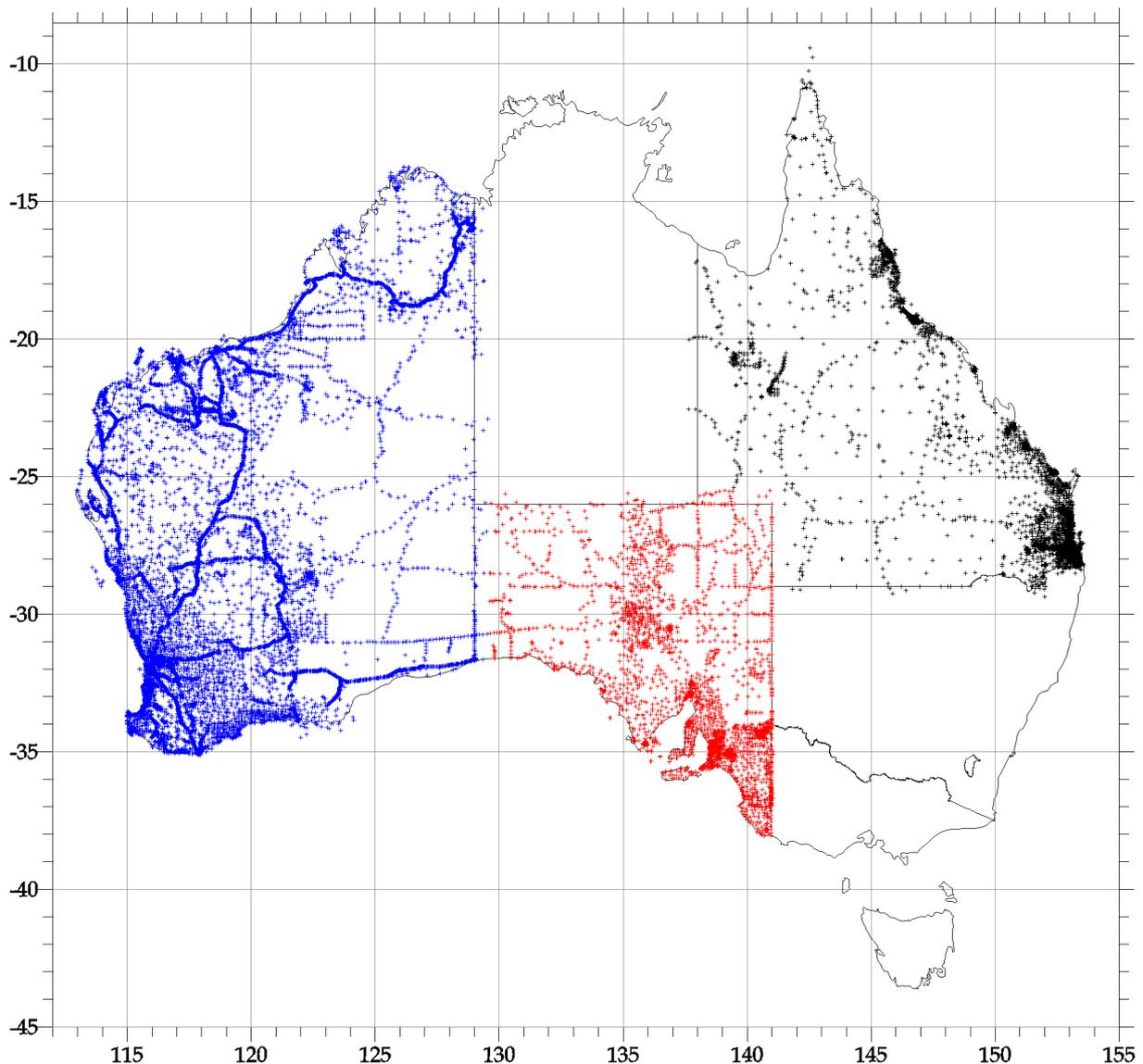
**Figure 11** – Distribution of data used to test the national AGD84 transformation grid
