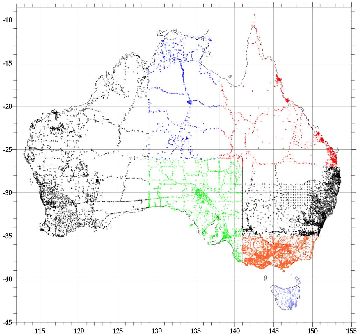
**Figure 14** – Distribution of data used to test the national AGD66 transformation grid
