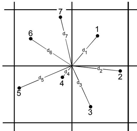
*Figure 3 – Interpolating distortion components at a grid node from surrounding data*
