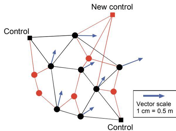
**Figure 2(b)** – Coordinate are re-calculated revealing distortion in original values
