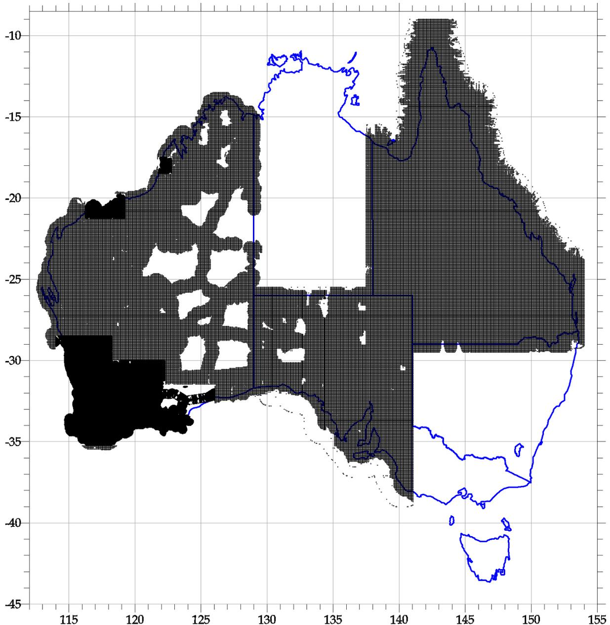
*Figure 12 – Conformal + distortion nodes in the national AGD84 transformation grid*
