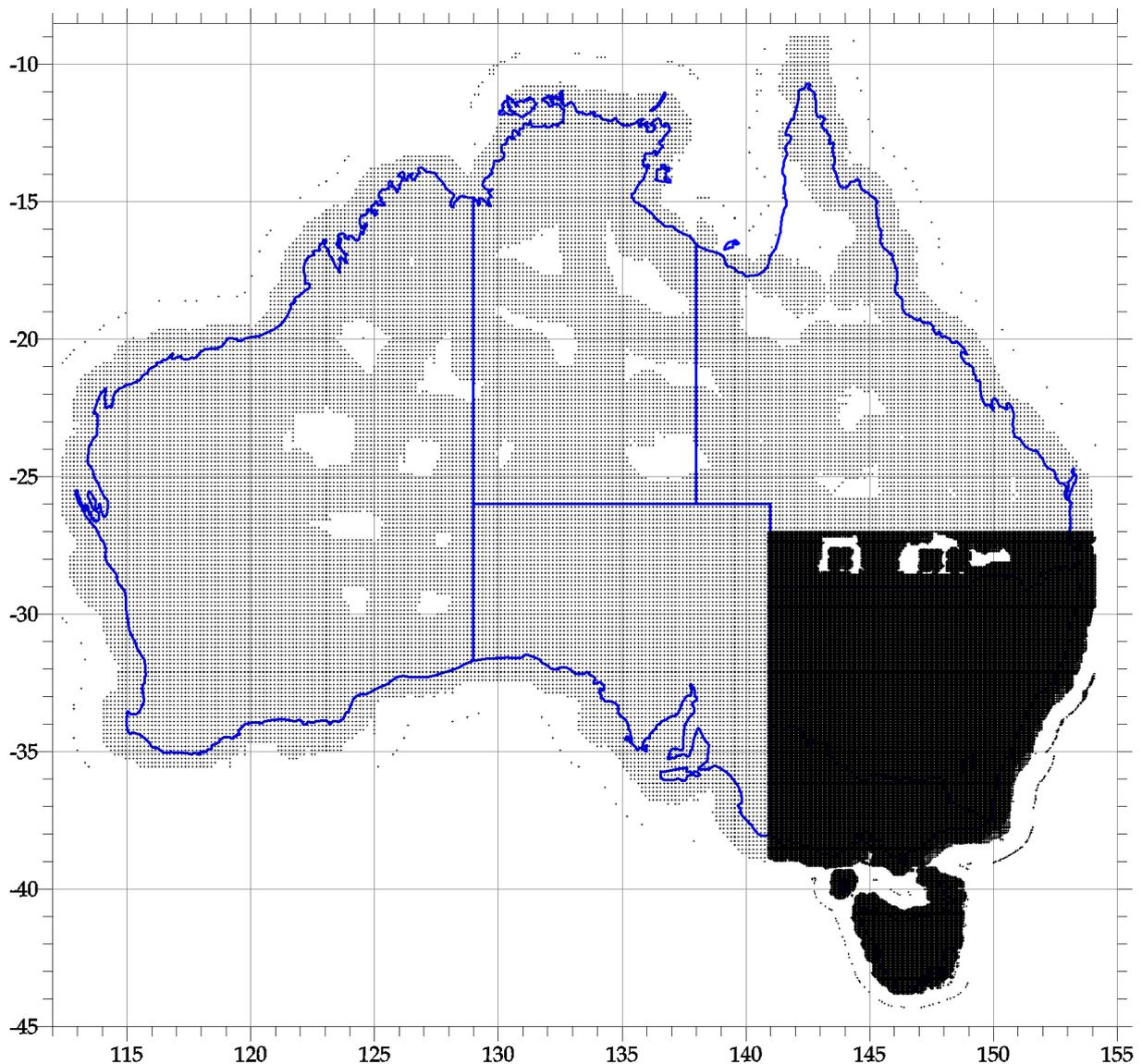
*Figure 15 – Conformal + distortion nodes in the national AGD66 transformation grid*
